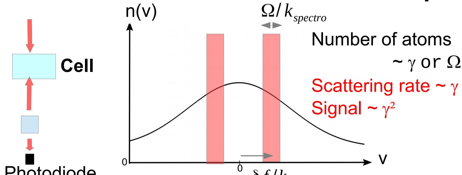
Saturated spectroscopy on the 7kHz-wide Sr intercombination line:
