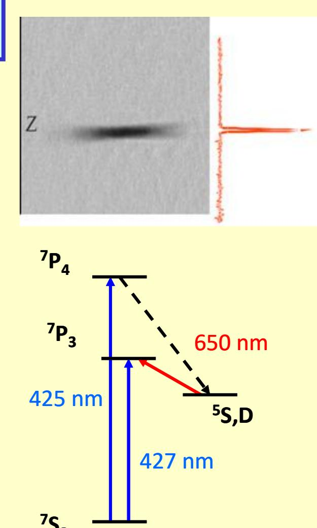
\*  $5 \times 10^6$  atoms fill the optical trap within 100 ms, @  $80 \mu\text{K}$ , density  $\sim 3.10^{11} \text{ at/cm}^3$ .
